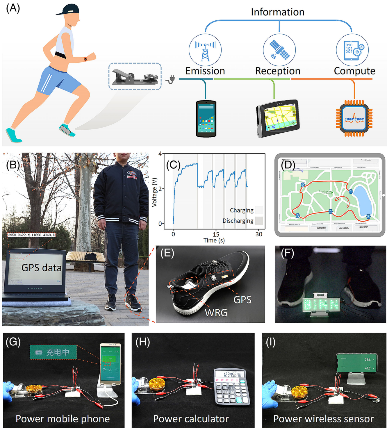
FIGURE 4 Applications of wearable noncontact free-rotating hybrid nanogenerator (WRG). A, Design the technical route of WRG. WRG could be utilized in information emission, reception, and compute. B-E, Application of a self-powered GPS system based on WRG. C, Charge curve of a capacitor ( 470 \mu\text{F} ) by WRG for GPS system. D, Image of the electronic map. E, Digital photograph of the self-powered GPS system. F, LEDs lighted up by WRG. G-I, Application as the universal power source for mobile phone, calculator charger, and wireless temperature sensor, respectively
