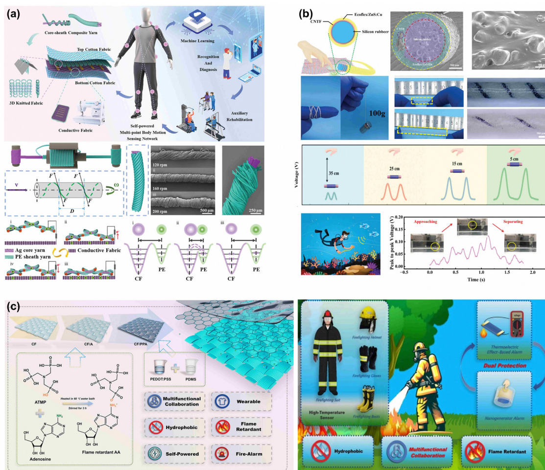
Fig. 8 Smart fabrics. (a) Structural design of a textile-based SMN and schematic diagram of a highly integrated gait recognition system. Schematic diagram of the manufacturing process and parameters of Ag-PE core-sheath composite yarn. Atomic-scale-electron-cloud potential-well model to describe the contact electrification between conductive fabric and PE sheath yarn. Reproduced with permission from ref. 154. Copyright 2023 Wiley-VCH GmbH. (b) Schematic diagram and SEM image of MLTENG principle. Photos of stretchable MLTENG and their corresponding optical images and dynamic loading structure diagrams. Output voltage of MLTENG at different distances and its application and transmission in water. Reproduced with permission from ref. 155. Copyright 2024 The Author(s). Advanced Science published by Wiley-VCH GmbH. (c) Illustration of the synthetic route of conductive fabric/polyphthalamide. Application of fire alarm system based on thermoelectric effect and TENGs. Reproduced with permission from ref. 156. Copyright 2024 Elsevier B.V. All rights are reserved, including those for text and data mining, AI training, and similar technologies.
