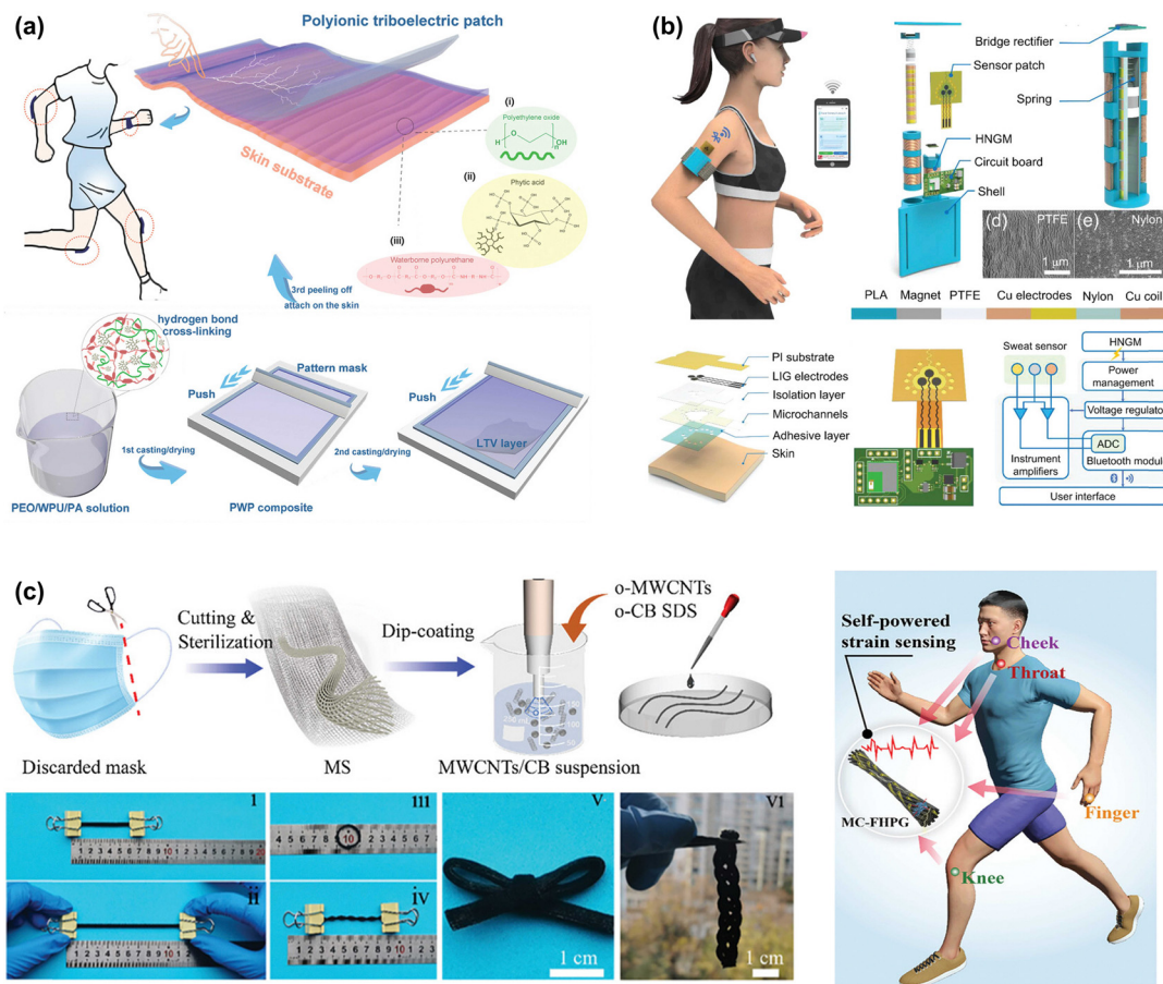
Fig. 9 Three cases of flexible devices. (a) Schematic illustration for the preparation of polyionic triboelectric patch. The patch structure consists of a polyethylene oxide/waterborne polyurethane/phytic acid current collector and silicon rubber tribolayer. Reproduced with permission from ref. 164. Copyright 2021 Wiley-VCH GmbH. (b) Schematics and structure diagram of the self-powered SWSAS for wireless molecular monitoring. Structural design of the HNGM. The SEM images of the etched PTFE and nylon film surface. Structure diagram of the sweat sensor patch. Reproduced with permission from ref. 89. Copyright 2022 Wiley-VCH GmbH. (c) Schematic illustration of the fabrication process for MC-FHPG. The stretchability, flexibility, and knittability of the MC-FHPG. Self-powered wearable strain sensing performance and human behavior monitoring applications. Reproduced with permission from ref. 168. Copyright 2023 Wiley-VCH GmbH.
