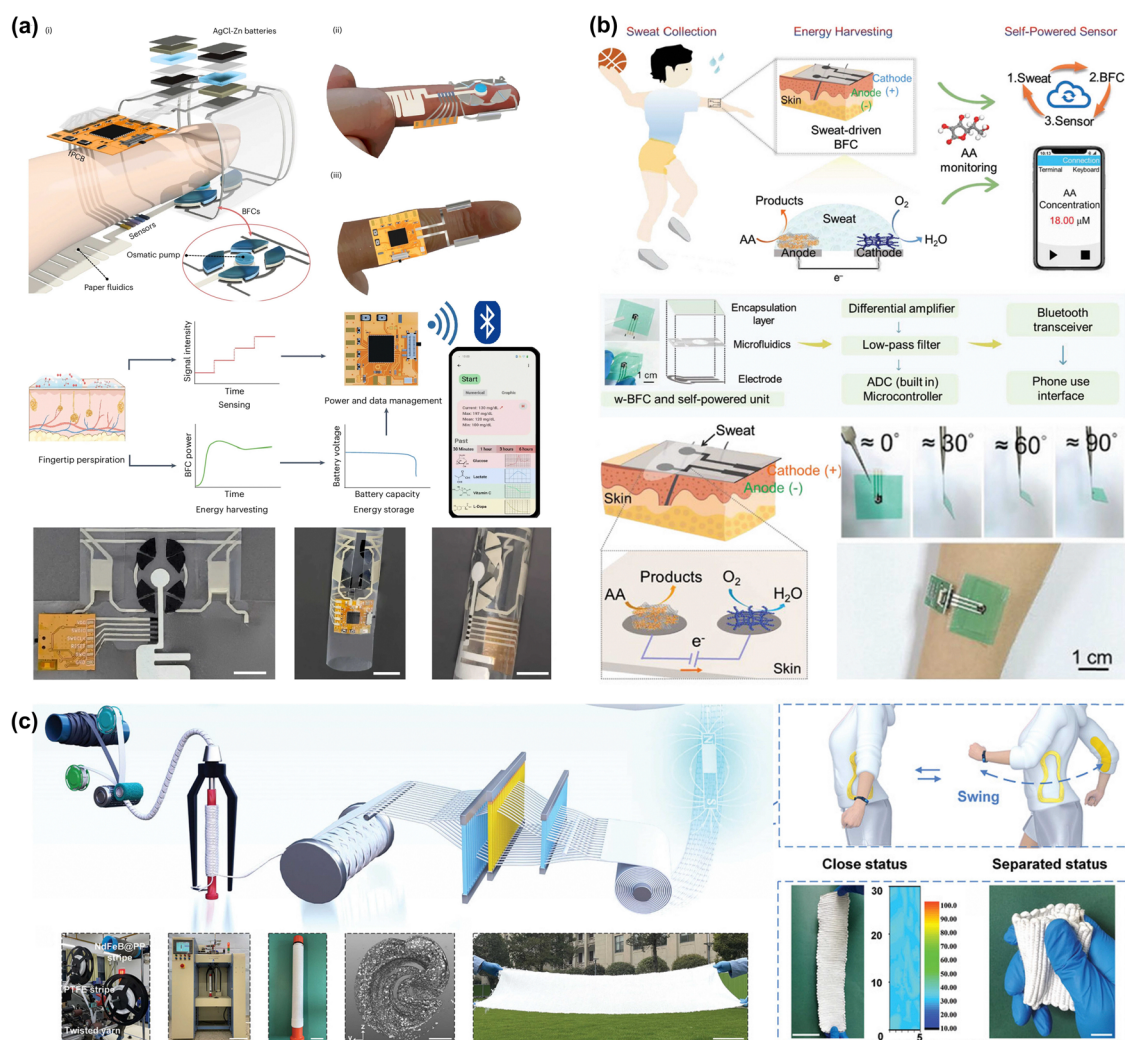
Fig. 6 The application cases of BFCs and magnetoelectric effect. (a) Schematic illustration of a fingertip-wearable microgrid system and its working principle, and optical image. Reproduced with permission from ref. 51. Copyright 2024, The Author(s), under exclusive license to Springer Nature Limited. (b) Schematic illustration of the metal hydrogel-based integrated w-BFC for sweat collection, energy harvesting, and self-powered sensor. Reproduced with permission from ref. 52. Copyright 2024 Wiley-VCH GmbH. (c) The process of preparing magnetic fabric. Microcomputerized tomography images of NdFeB magnetic yarn. A piece of 1 \times 3 \text{ m}^2 plain weave fabric formed by industrial weaving machines. Physical photograph and magnetic field distribution of 5 \times 30 \text{ cm}^2 magnetic fabric with good flexibility and foldable softness. Reproduced with permission from ref. 127. Copyright 2021 Wiley-VCH GmbH.
